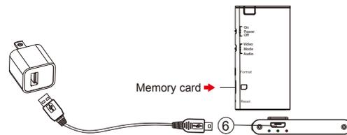
Plug the micro USB end of cable into USB port (6) and plug the other end to an USB power source. After charging, with golden contact facing down, insert the memory card into the card slot (4). Then the device will be ready for further operations.
