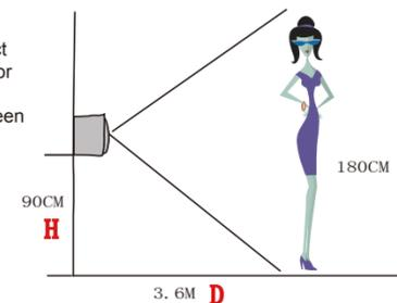
For example: To film a man at 180cm height in the video, the sensor should be placed at 90cm height above the ground and the man is 3.6m away from the sensor.
