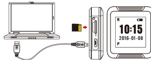
Plug the micro USB end of cable into USB port and plug the other end into the computer or other USB power source. After charging, with golden contact facing up, insert the memory card into the card slot. Then the device will be ready for further operations.
